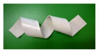
MasterSeal 528 is reinforced with a unique inorganic natural non-toxic high aspect ratio microfibers (length / diameter), able to create a micro three-dimensional homogeneously diffused reinforcement to improve the crack bridging ability and tensile strength of the waterproofing membrane.
