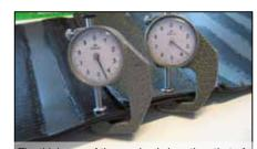
The thickness of the overlap is less than that of the strips, which ensures maximum stability for the insulating panels laid across the overlap.
