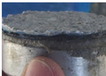
2.6 Heavy weight fabrics form bundles of filaments which the adhesive cannot penetrate (left: 1200 gsm fabric, right: 800 gsm fabric)
